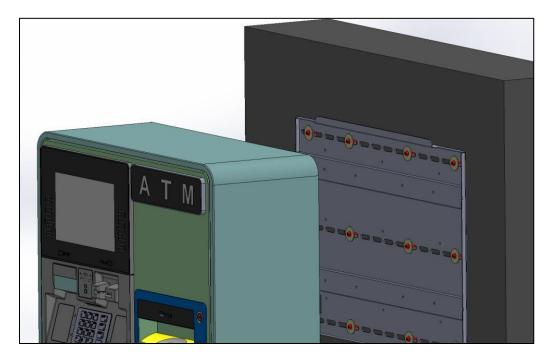
With the machine installed on the mounting bracket, you can now open the front of the machine to access the 8 screws that will be used to secure the machine to the bracket.
