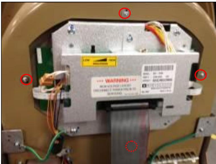
9b. Re-attach the green grounding straps on the left and right sides of the rear of the Monitor.
