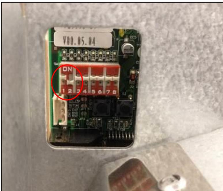
If the Receipt Printer Control Board has only 2 Dip Switches, set Dip Switch 1 to the OFF position and Dip Switch 2 to the ON position.
