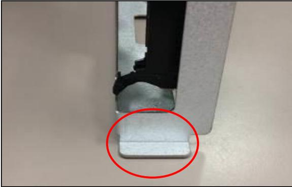
8b. Align the grounding straps and, utilizing the two retained screws, attach the housing to the ATM as shown.
