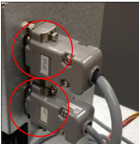
6b. Disconnect all of the cable connections at the rear of the Main Control Board. The new Main Control Board comes with the required cable connectors to attach internal cabling that will remain in the ATM. You will also need to disconnect the RJ11 phone cable from its connection at the top rear of the Modem.
