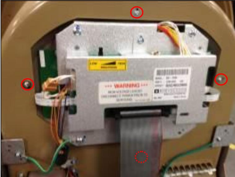
6. Remove the existing Main Control Board
