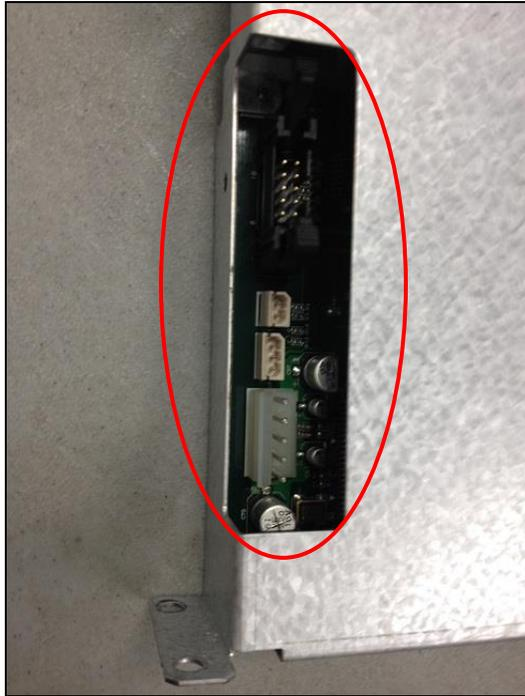
6c. The Main Control Board and metal housing is attached to the ATM with two screws at the rear base. Green grounding straps are attached at this same location. Remove the two screws (and retain). The Main Control Board and housing can now be lifted and removed.
