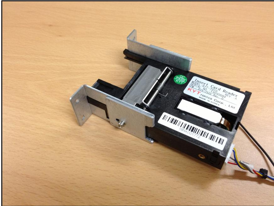
Using the 4 course-thread screws included with the kit, install the new reader assembly into the back of the card reader bezel.
