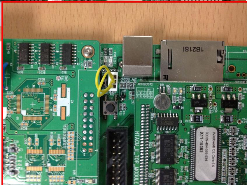
Once the jumper has been installed, you're ready to reinstall the cover over the motherboard and verify that all the wires are attached properly.
