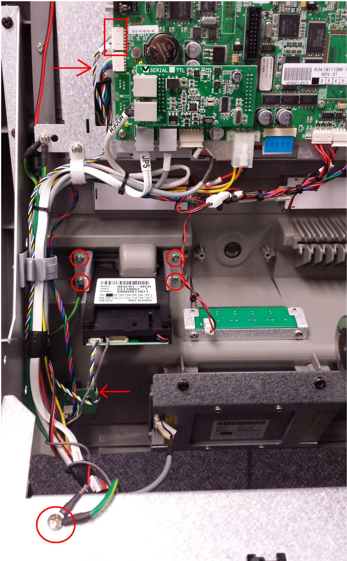
Once the cable is freed up, remove it from the ATM completely along with the card reader. You will not reuse either of these.
