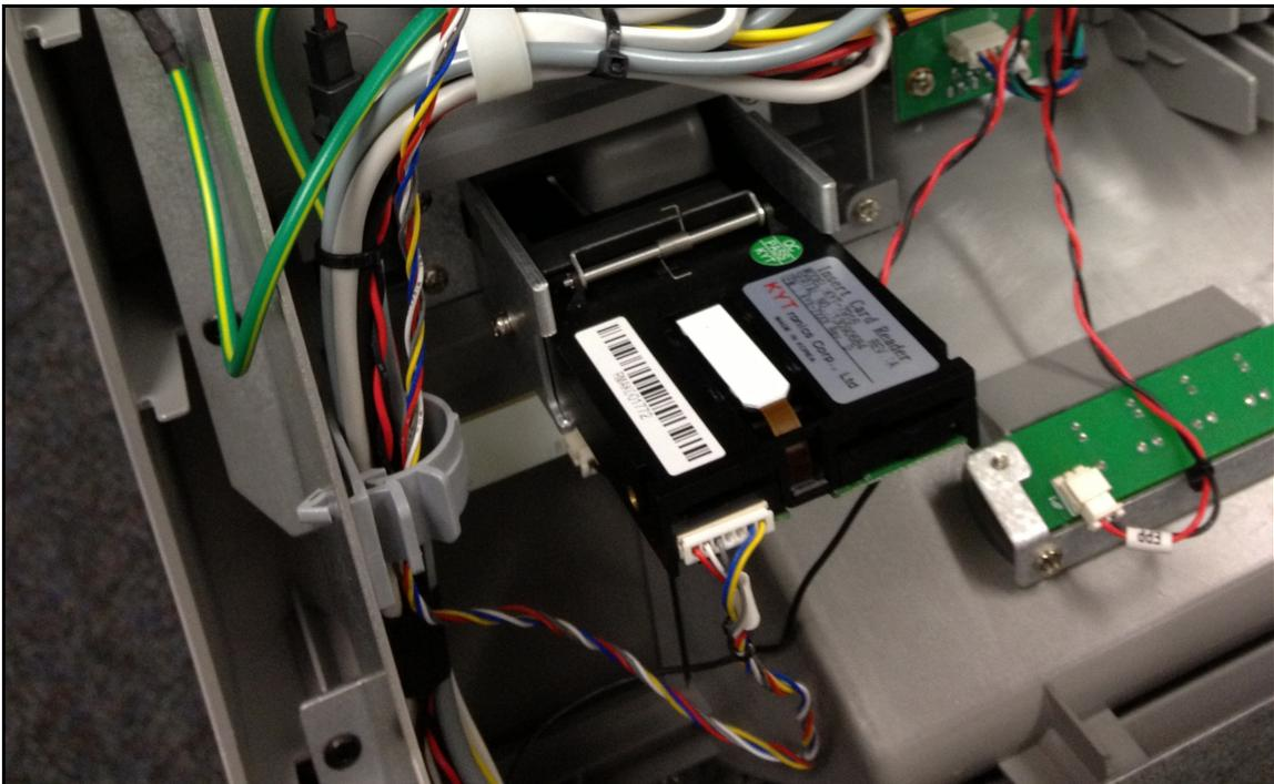
When you install the new card reader, we recommend leaving the screws a little loose, and then try inserting a card in from the front. The card should slide in and out easily without hanging up on the bezel.
