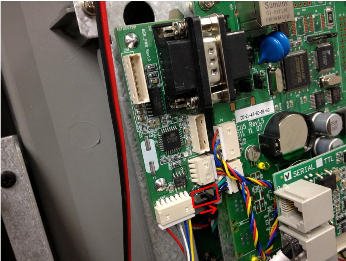
Plug the jumper wire in as shown above, the wires will be tight, so route them down under the modem so they do not get pinched. Attach the card reader wire to the bottom.
