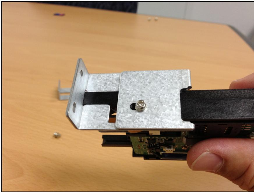
With both brackets installed as shown, you're ready to install the assembly to the back of the bezel.
